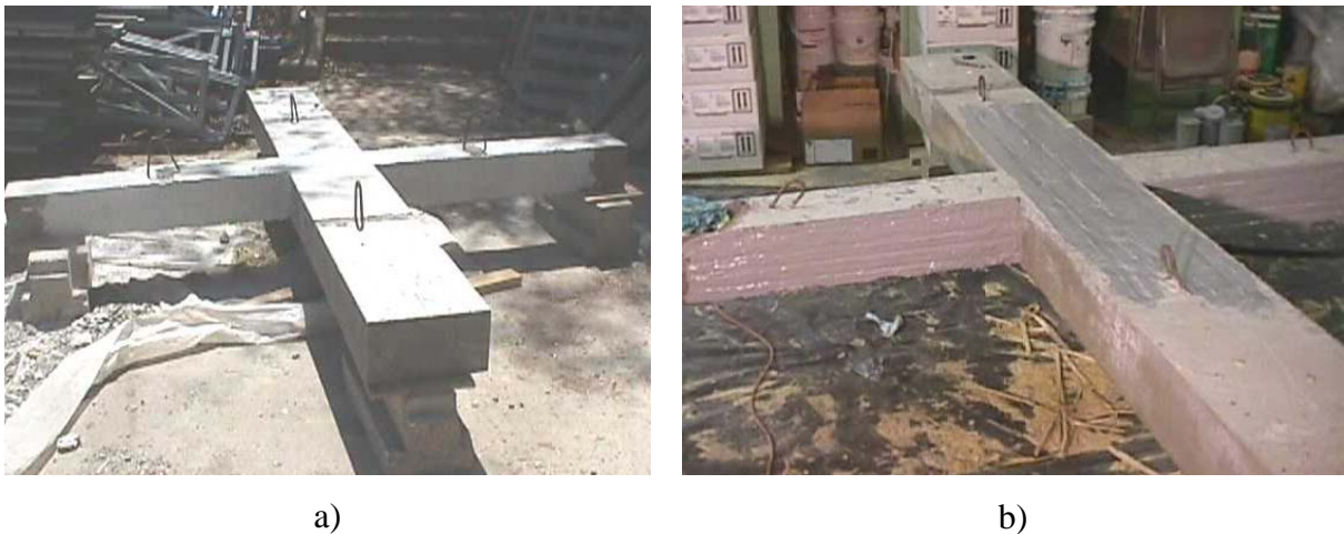
Figure 3. 2 NSM rods in the columns (a) and joint (b)
