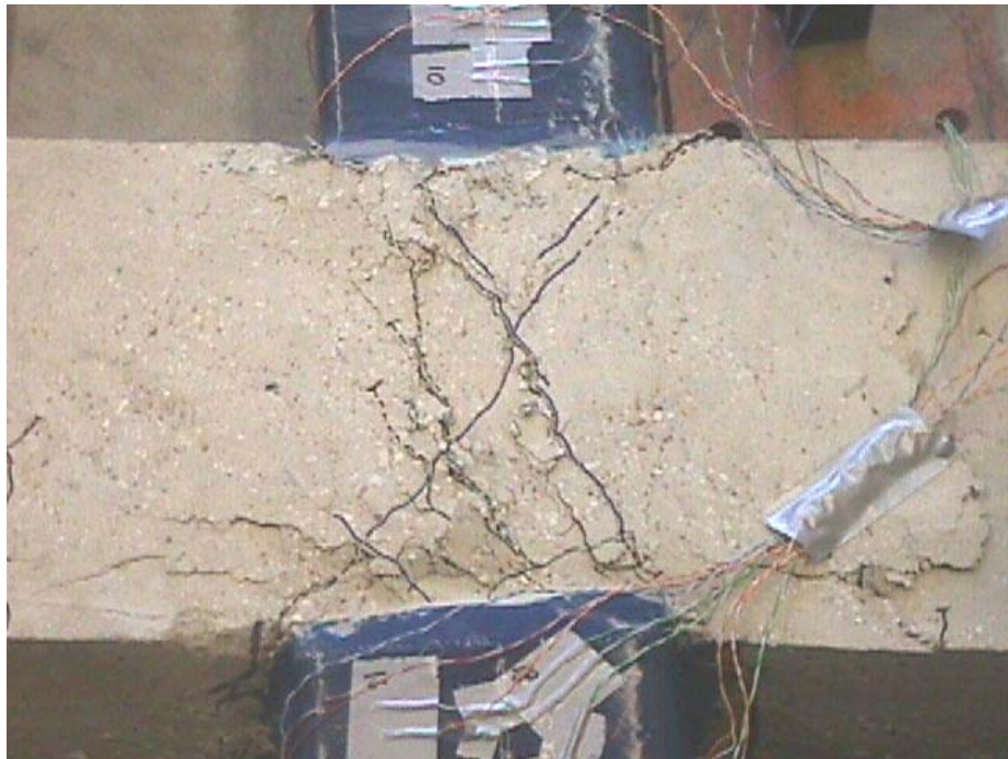
Figure B. 42 Top view of shear failure of the panel: joint L3
