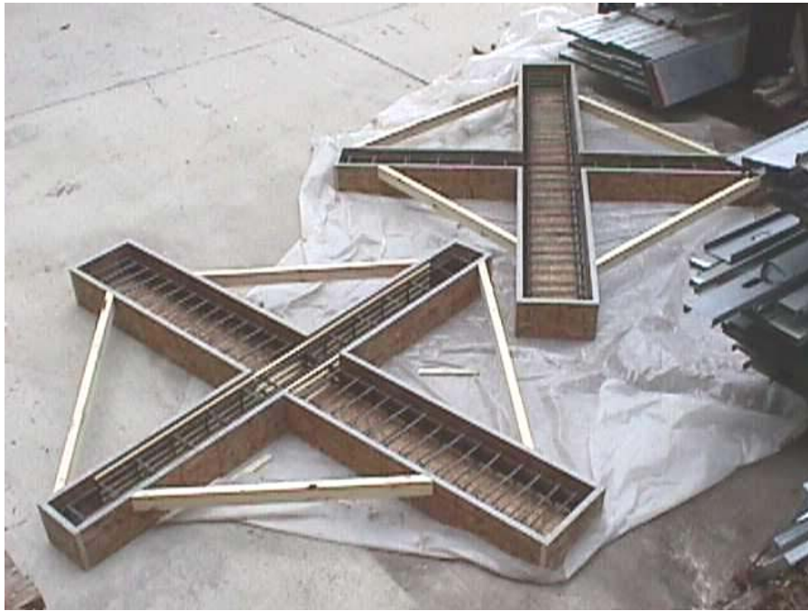
Figure A. 1 Typical formworks: on the left H3, on the right H1
