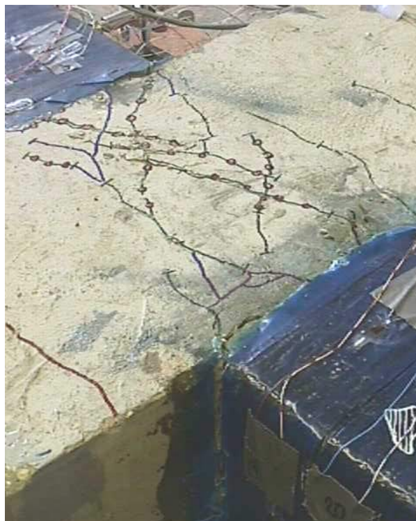
Figure B. 35 Tension failure of column: joint H2U
