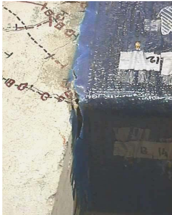
Figure B. 34 Tension failure of column: joint H2
