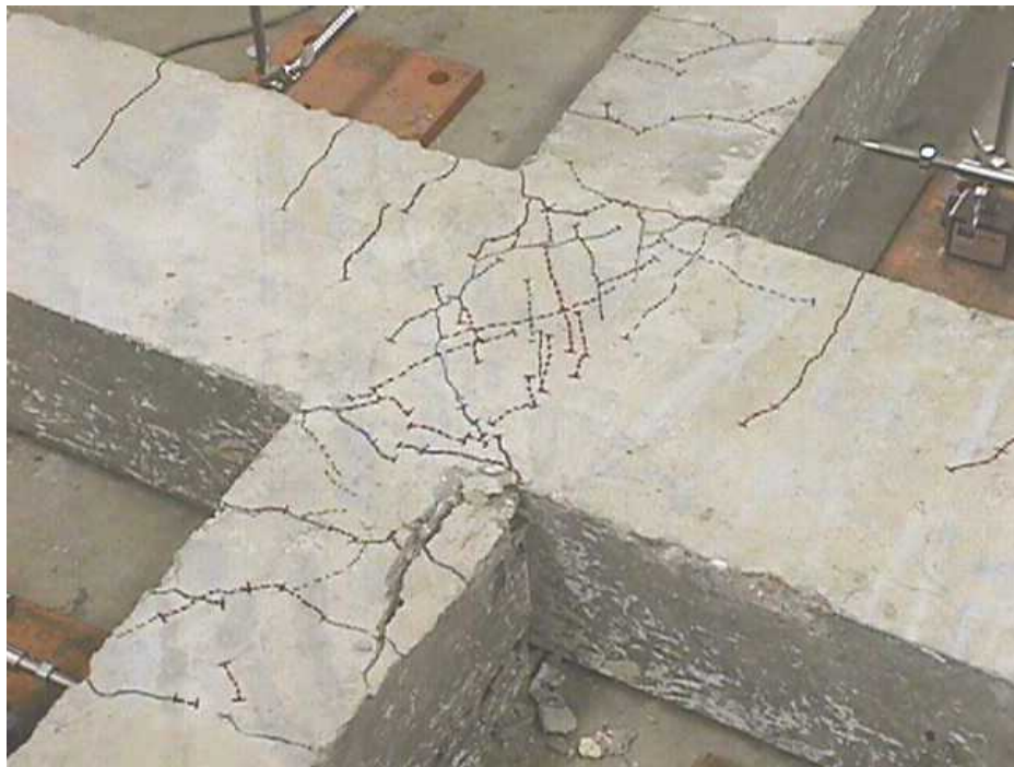
Figure B. 12 Crack pattern at failure: joint L1
