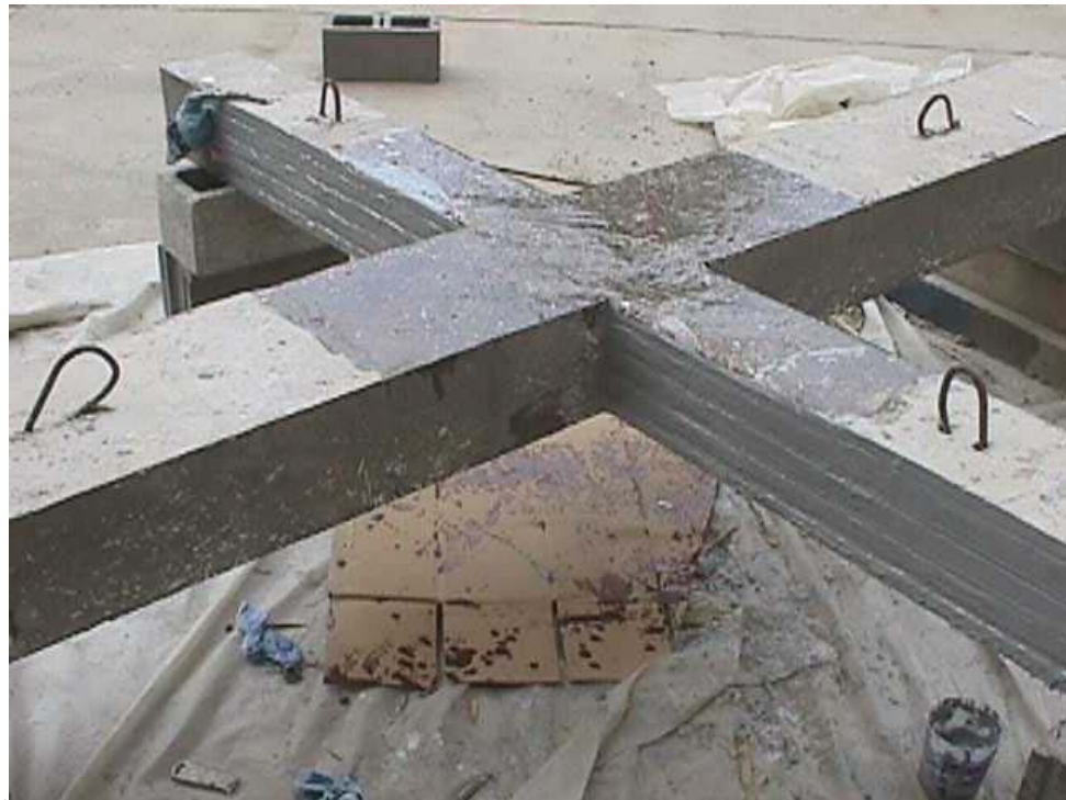
Figure A. 28 Curing of the primer prior to putty application
