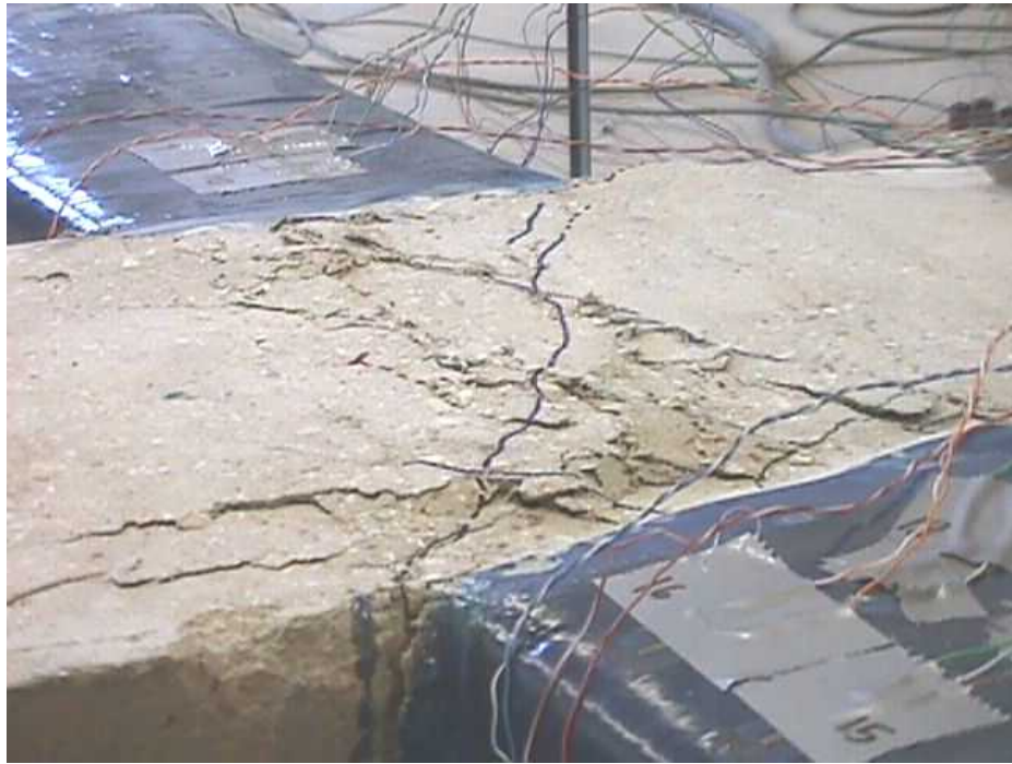
Figure B. 43 Shear failure of the panel: joint L3
