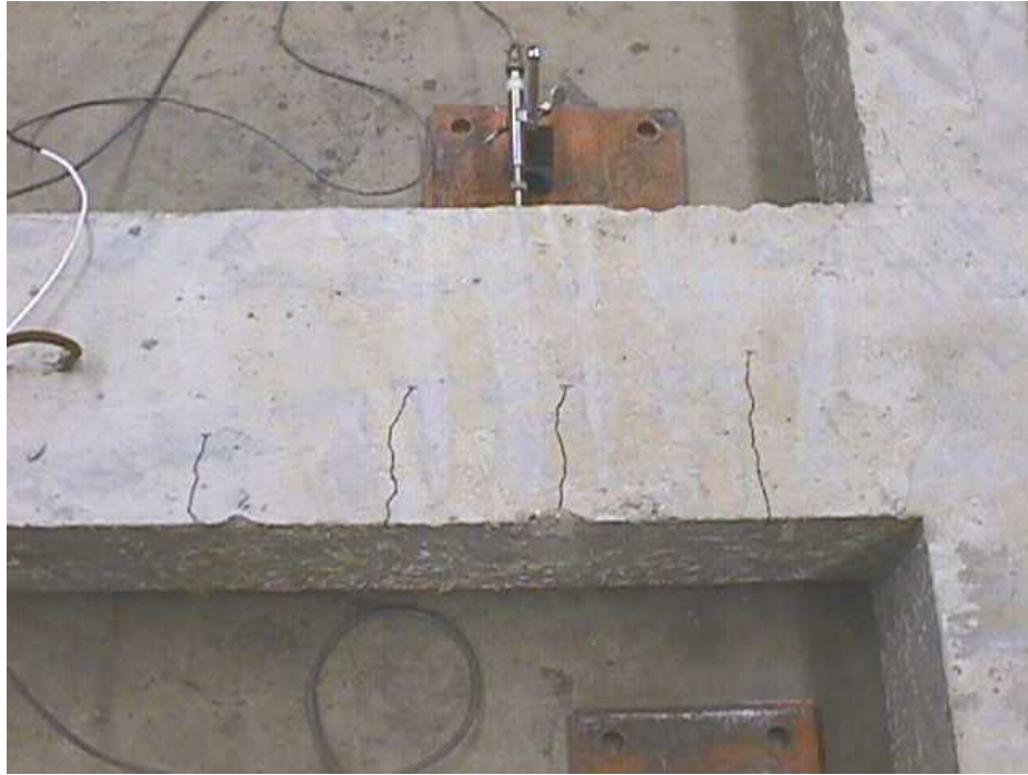
Figure B. 5 Initiation of flexural cracks in the beam: joint L1
