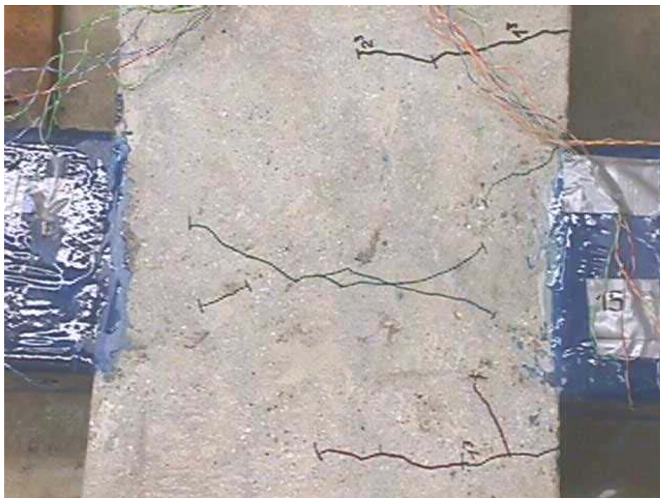
Figure B. 26 Initiation of shear cracks in the panel: joint H2L
