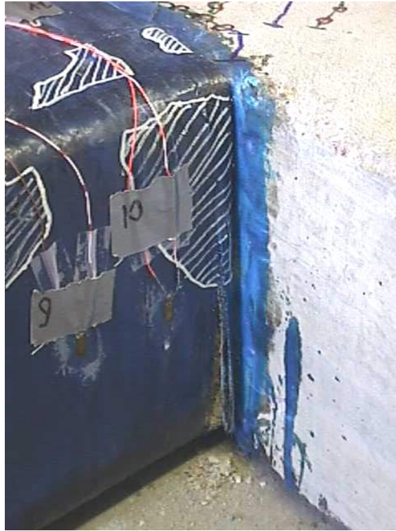
Figure B. 36 Combined panel-column failure: joint H2
