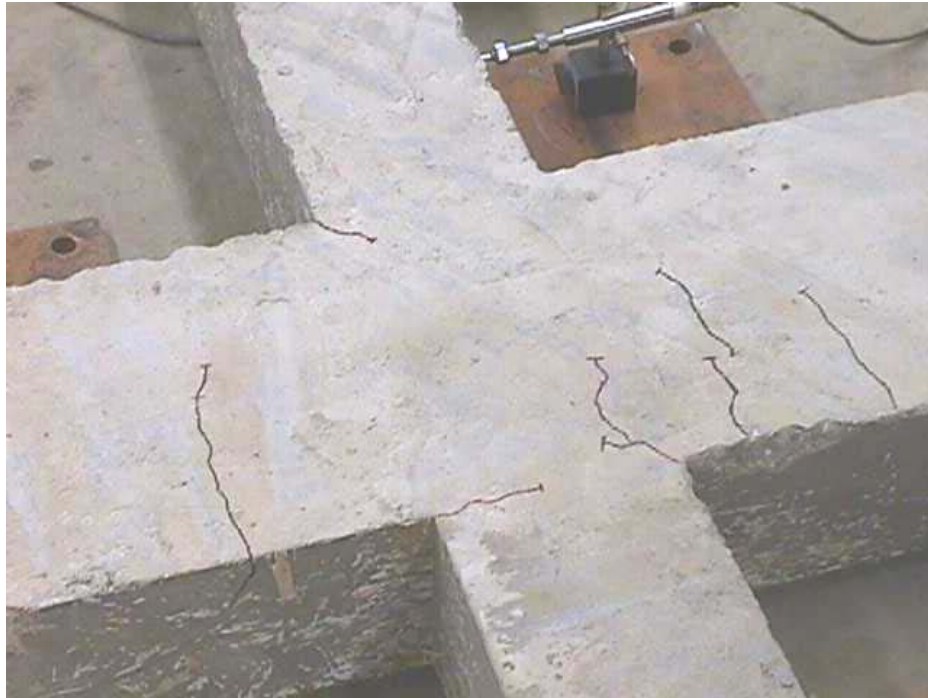
Figure B. 7 Initiation of shear cracks in the panel: joint L1
