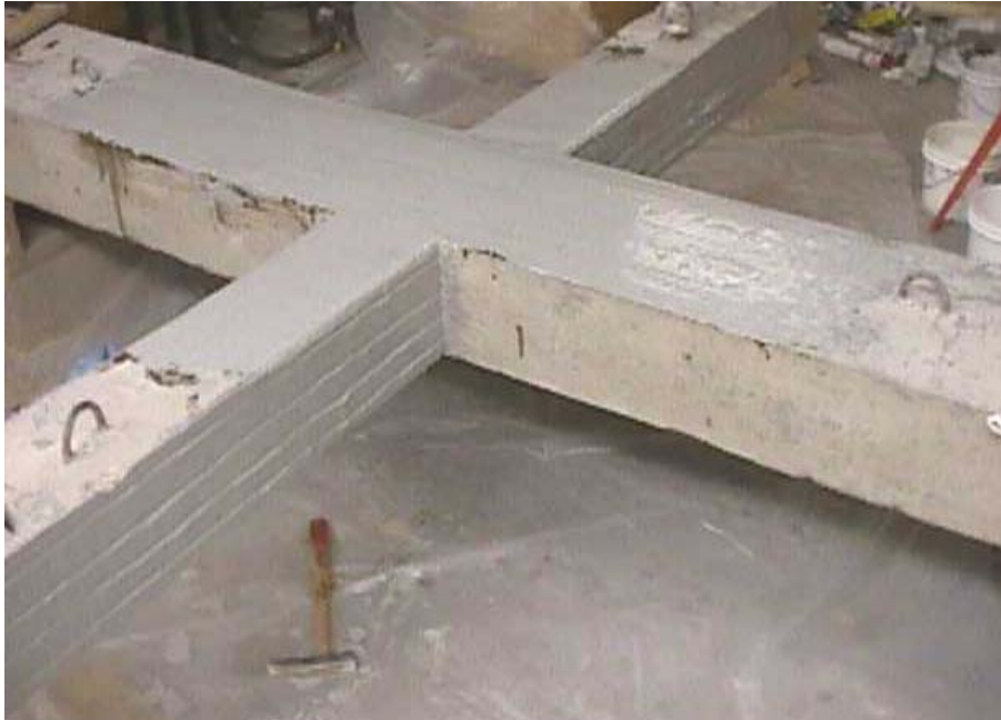
Figure A. 25 NSM rods installed into the columns and the panel
