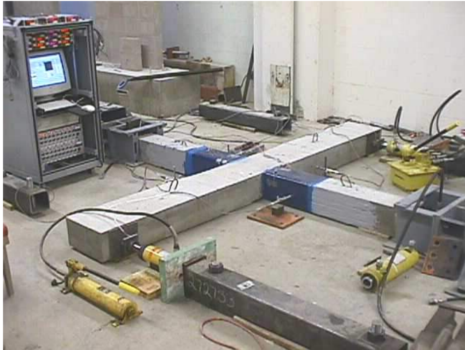
Figure B. 3 Test setup view from the superior column
