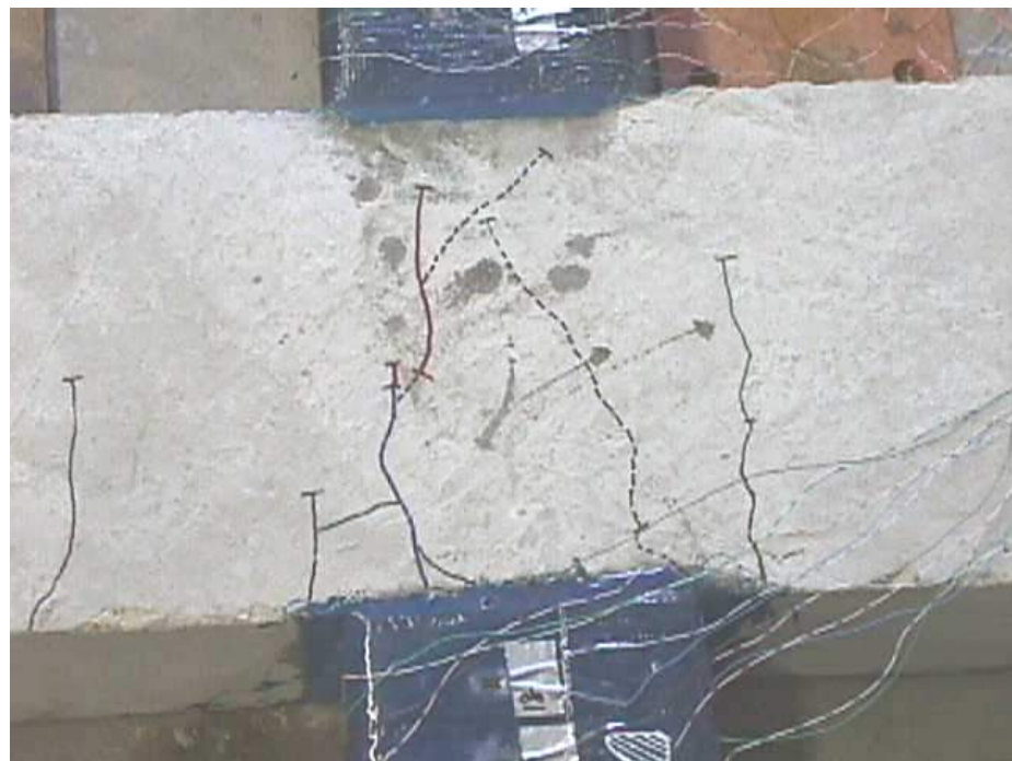
Figure B. 28 Initiation of diagonal cracks in the nodal zone: joint H2U
