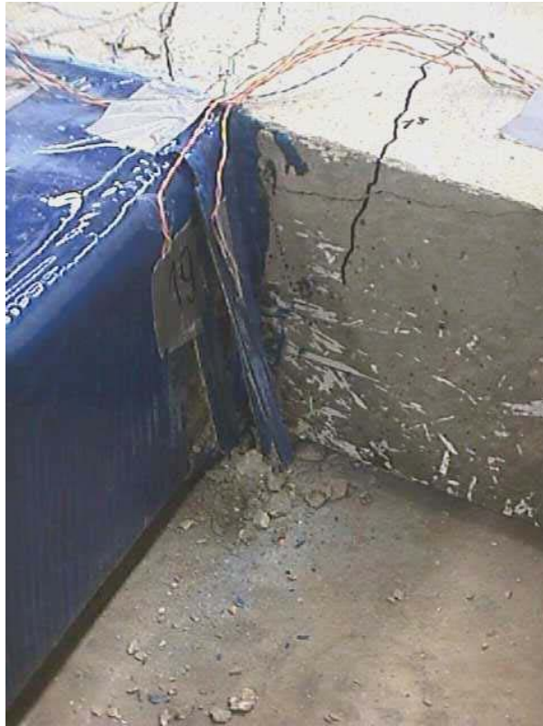
Figure B. 38 Shear failure of the panel: joint H2L
