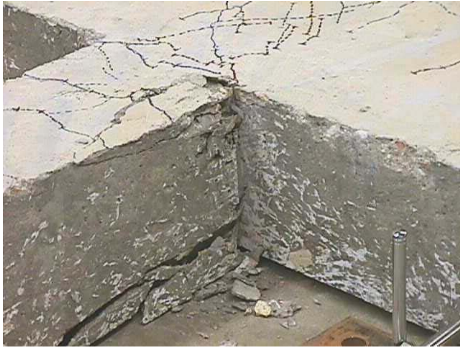
Figure B. 11 Lateral view of failed column: joint L1
