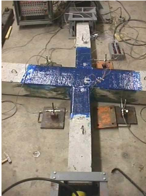
Figure B. 50 Separation at panel-inferior column: joint L4
