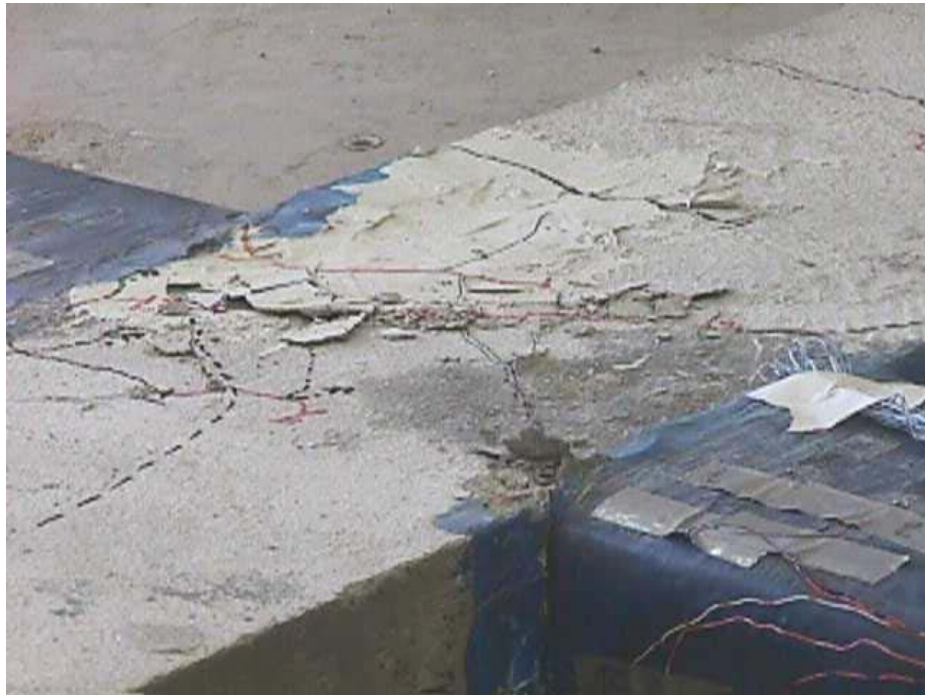
Figure B. 45 Damage due to panel shear failure: joint H3
