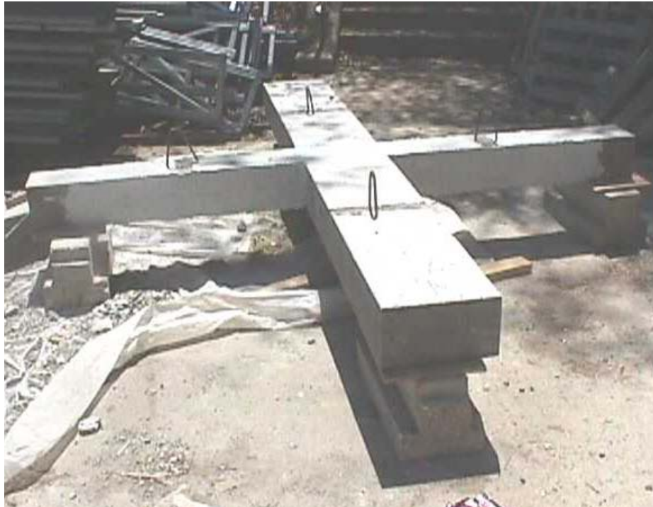
Figure A. 23 Joint after installation of NSM rods has been completed
