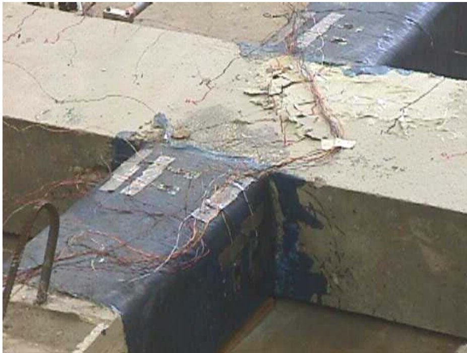
Figure B. 44 Shear failure of the panel: joint H3
