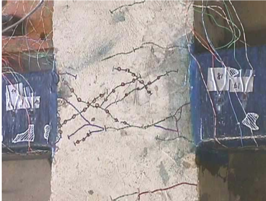
Figure B. 25 Propagation of diagonal cracks in the nodal zone: joint H2
