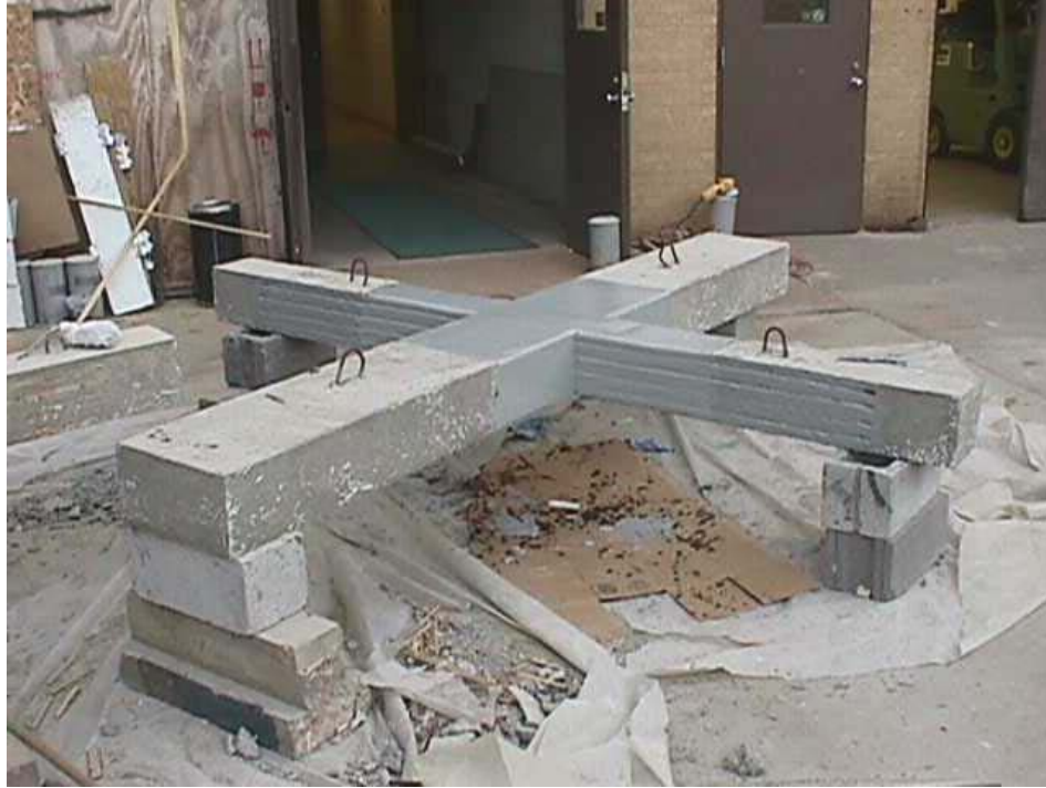
Figure A. 29 Curing of putty prior application of saturant
