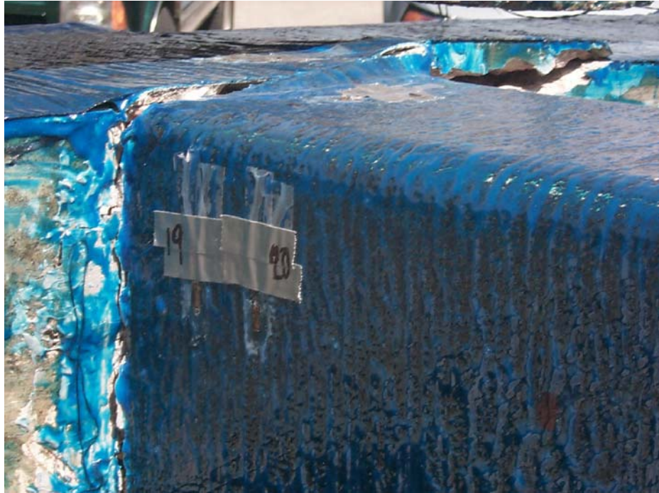
Figure B. 48 Separation at panel-superior column: joint L4
