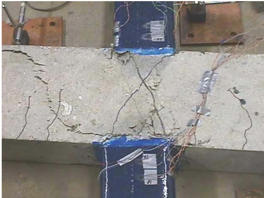
Figure B. 46 Panel shear failure: joint M3
