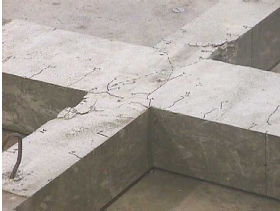
Figure B. 17 Failure of the columns: joint H1
