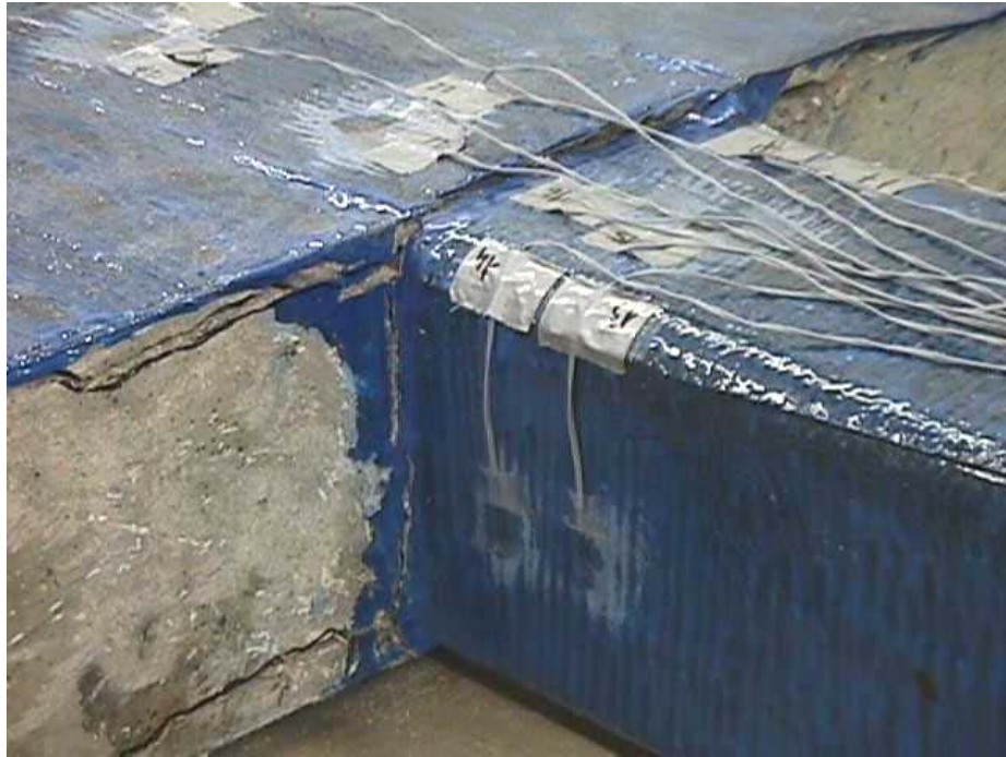
Figure B. 56 View from the superior column at failure: joint H5
