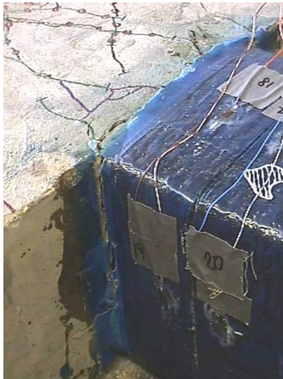
Figure B. 33 Panel damage: joint H2U
