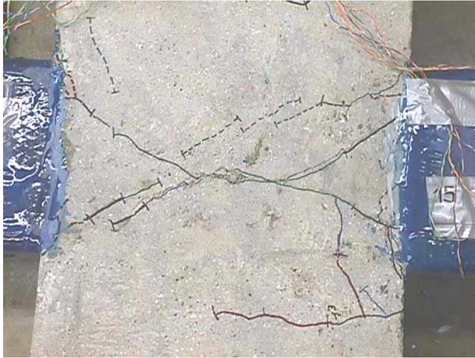
Figure B. 27 Propagation of shear cracks in the panel: joint H2L
