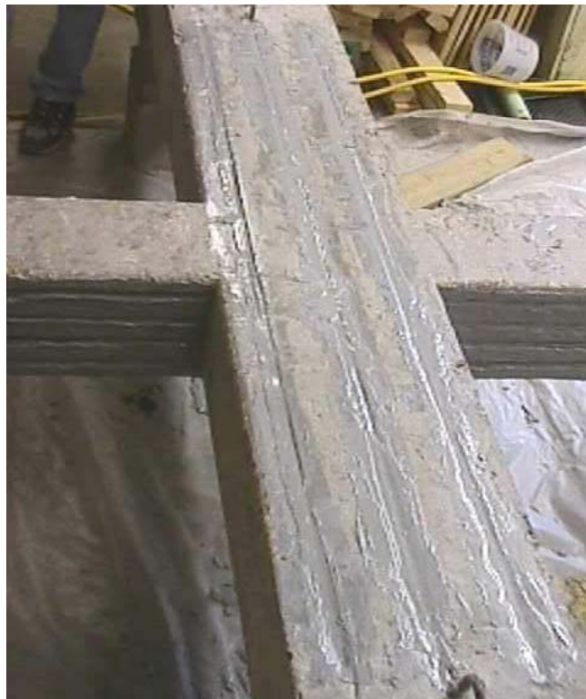
Figure A. 24 NSM FRP rods as horizontal reinforcement of the panel
