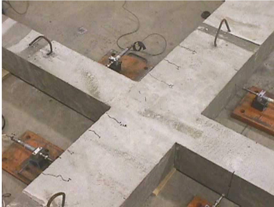
Figure B. 13 Flexural cracks in the beams: joint H1
