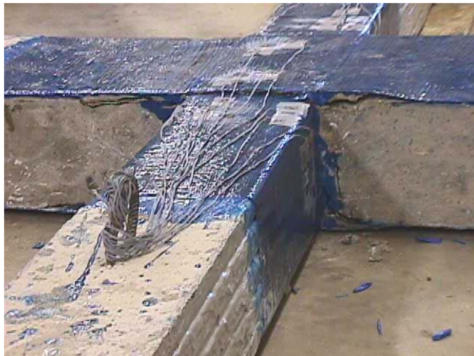
Figure B. 55 Separation at panel-inferior column: joint H4
