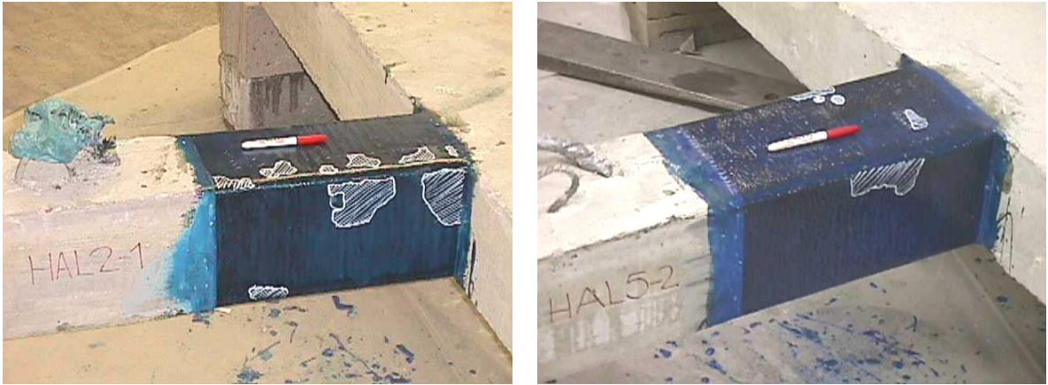
Figure 3. 9 Monitored debonding zones on specimens H2 and H2U
