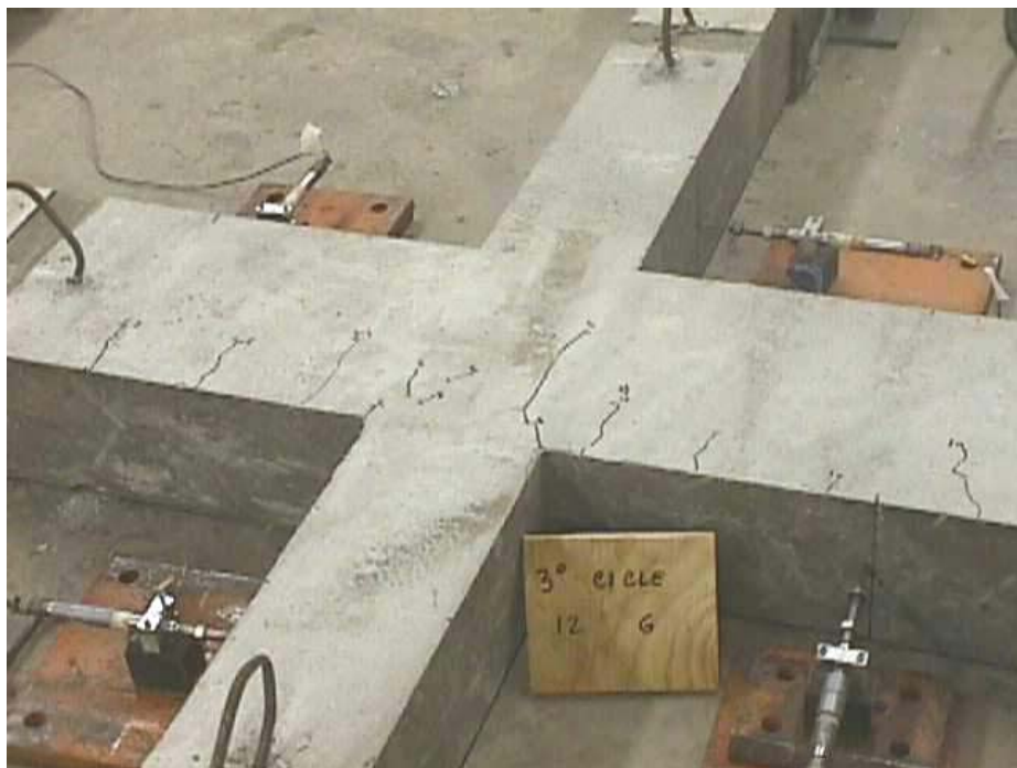
Figure B. 14 Initiation of shear cracks in the panel: joint H1
