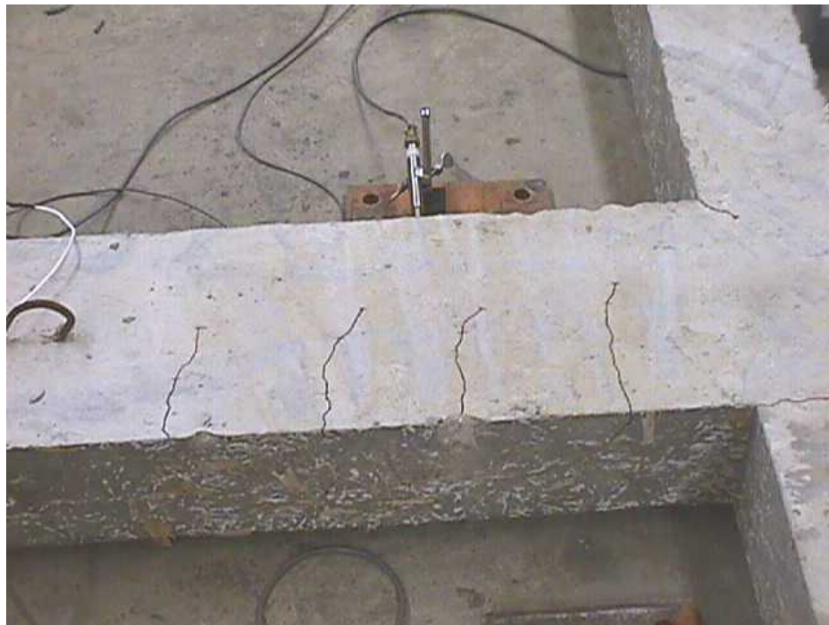
Figure B. 6 Propagation of flexural cracks in the beam: joint L1
