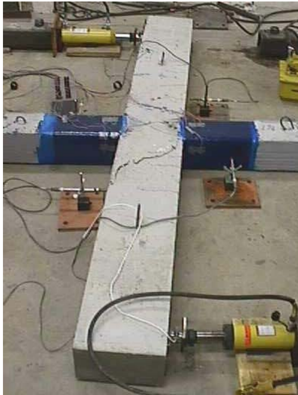
Figure B. 47 Top view of joint M3 at failure
