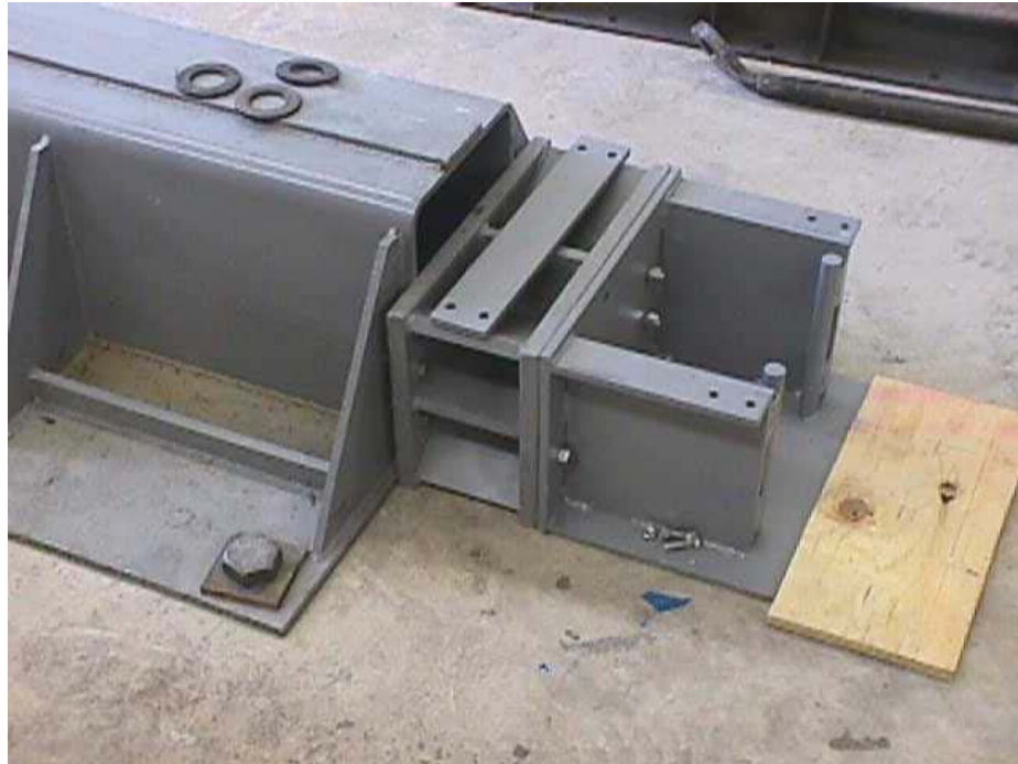
Figure B. 1 Restraint at the column end
