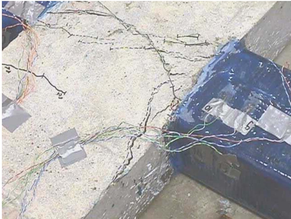
Figure B. 37 Initiation of fibers breaking in column compression region: joint H2
