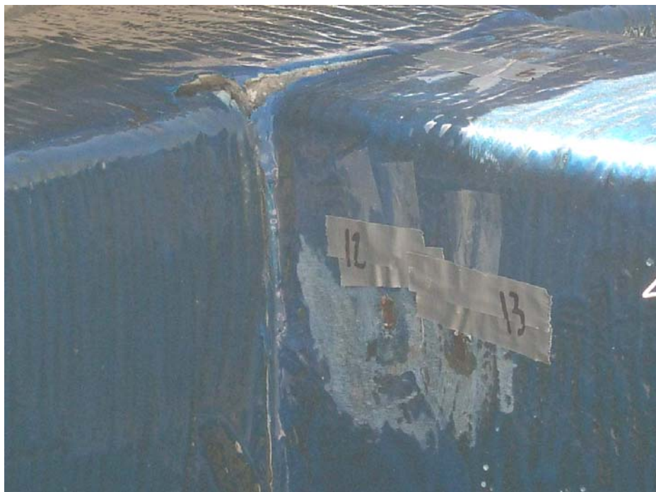
Figure B. 49 Lateral view of the superior column at failure: joint L4
