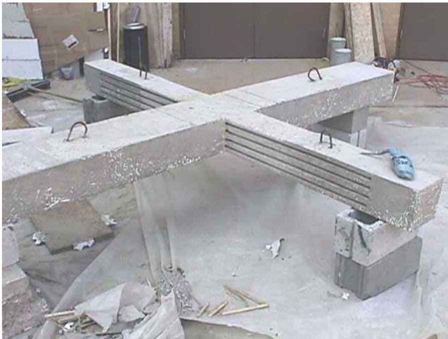
Figure A. 16 Joint prepared for the installation of NSM rods
