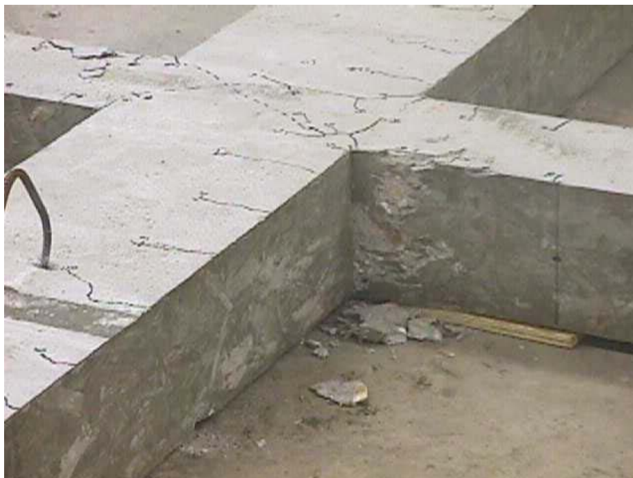
Figure B. 16 Lateral view of failed column: joint H1
