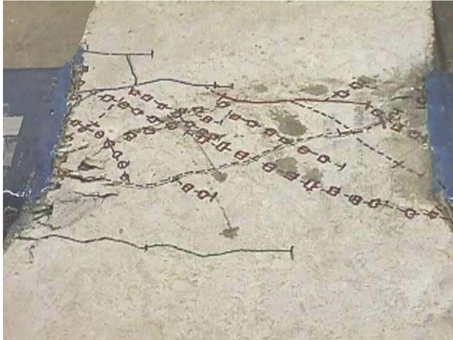
Figure B. 33 Panel damage: joint H2U
