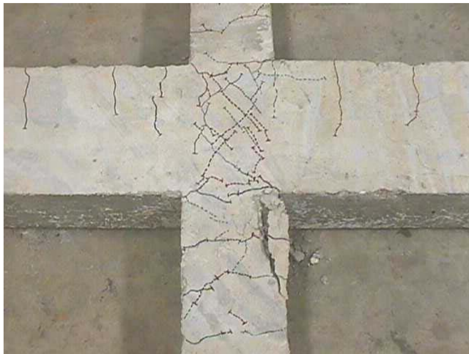
Figure B. 10 Column failure: joint L1
