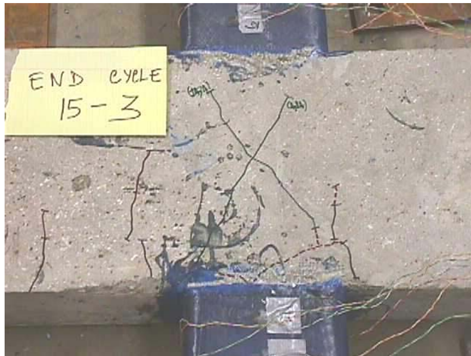
Figure B. 19 Initiation of shear cracks in the panel: joint L2
