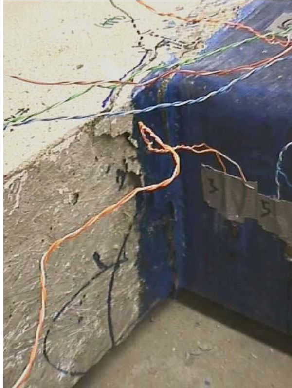
Figure B. 23 Lateral view of failed column: joint L2
