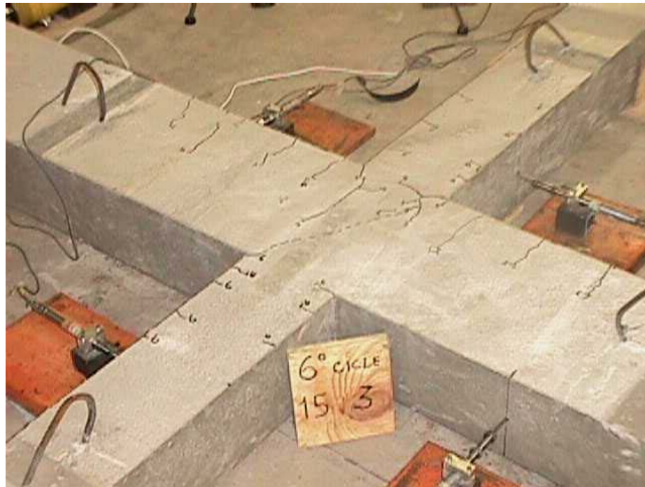
Figure B. 15 Opening of flexural cracks in the columns: joint H1
