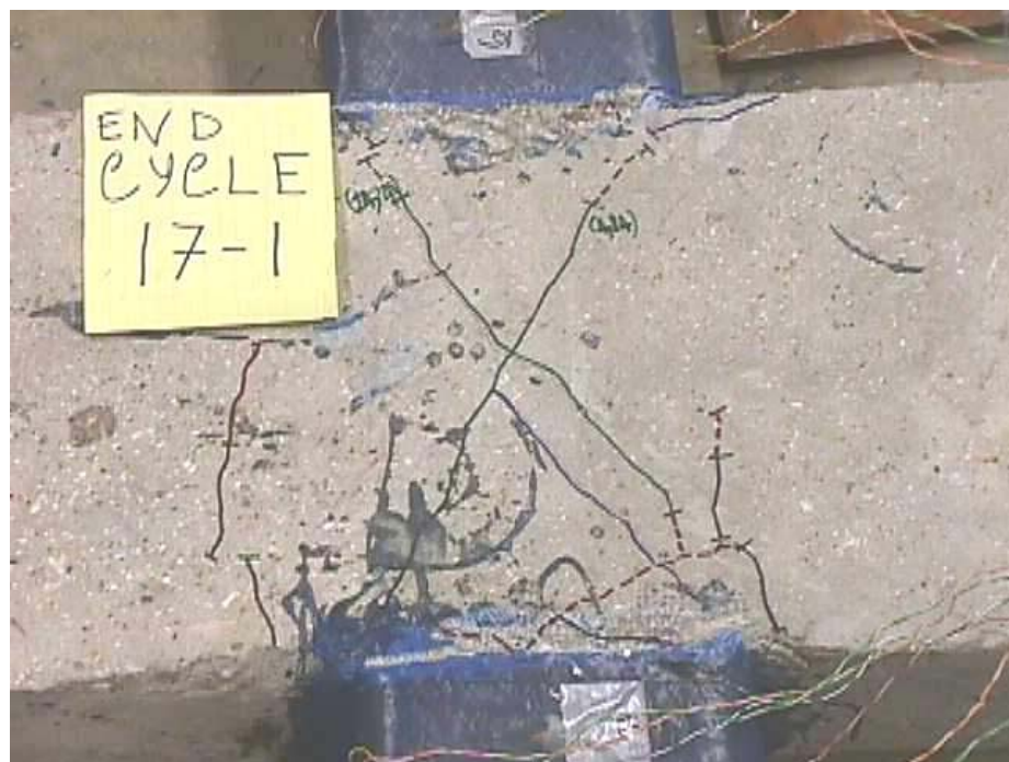
Figure B. 20 Propagation of shear cracks in the panel: joint L2
