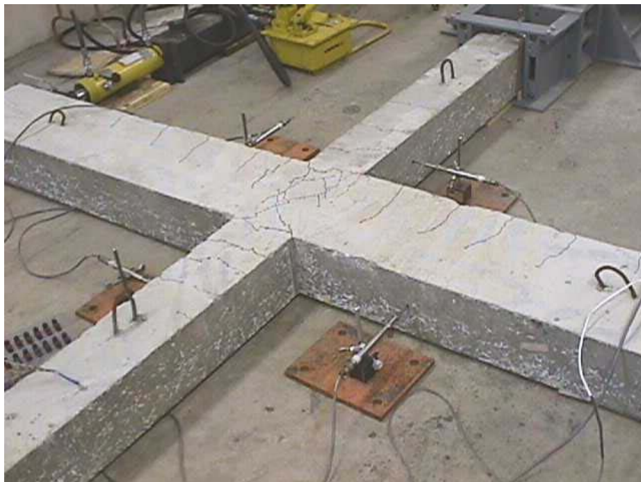
Figure B. 4 LVDT transducers on both columns and beams
