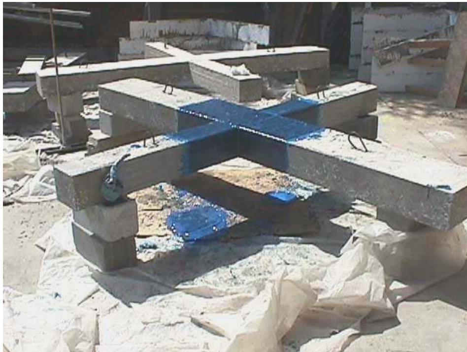
Figure A. 30 U-wrapping of beam around its bottom surface: joint H5
