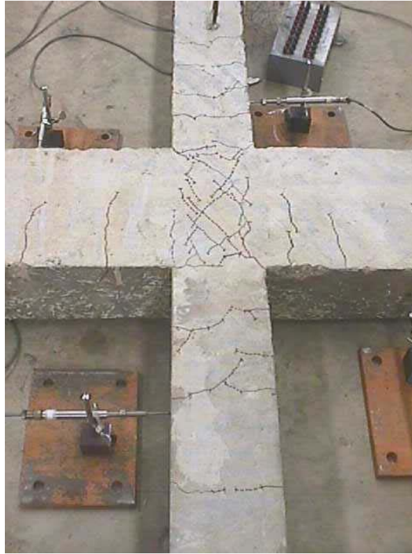
Figure B. 9 Propagation of shear cracks in the panel: joint L1
