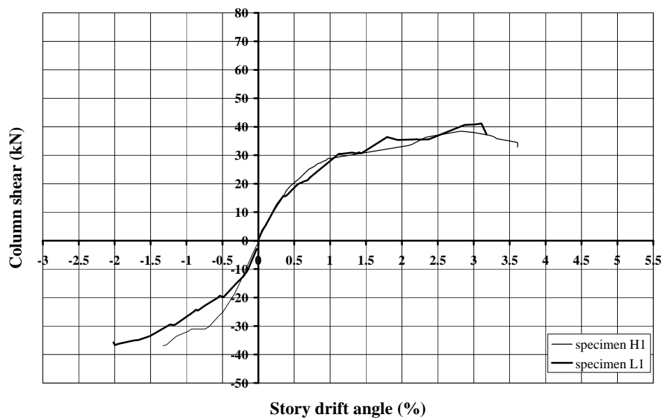
Figure C.50 Column shear-story drift: comparison for type 1 connections
