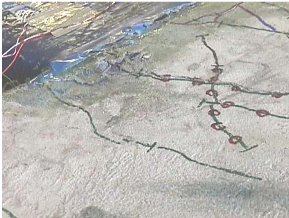
Figure B. 30 Panel damage: joint H2
