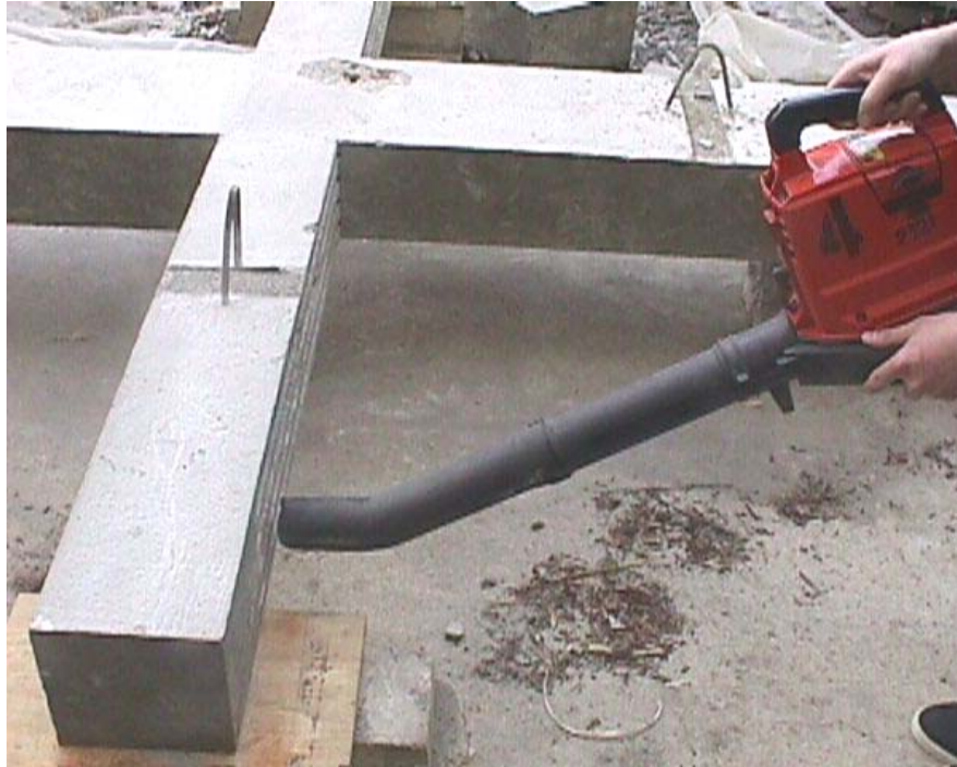
Figure A. 17 Blowing of the grooves
